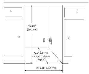
\* Depth dimension may vary depending on each individual installation. A minimum depth of 27-1/2" (69.9cm) is required with ample provision for wiring.
