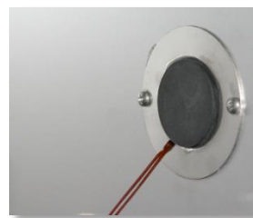
Figure 16: Introducing a sensor probe through the access port.
