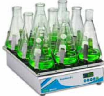
Orbi-Shaker™ Orbital Shaker by Benchmark Scientific Powerful motor drive able to shake a 14 lb. load at up to 300 rpm
