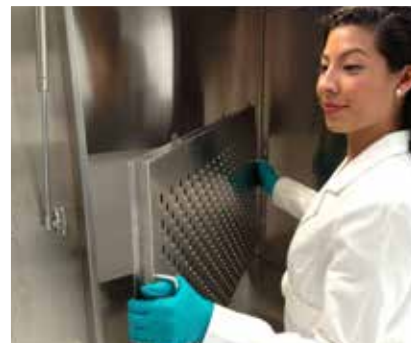
Rear Baffle removes for cleaning
